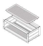
A cover plate is used for electromagnetic shielding or as mechanical protection. The cover can be screwed onto the side panel. Can be used for railway subracks in accordance with SNCF.
