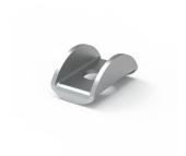
This busbar saddle, MSBC, has been tested according to IEC 61439 and is available off the shelf. It is easy to mount and connects two bars with a thickness of 10 mm, to enable the connection of an electrical cable.
