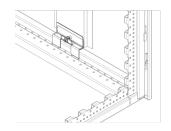
The internal retainer is easily fitted without drilling, and allows the rear panel to be removed only from inside. The retainer is only for IP 20 applications.
