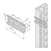
DIN rail for thermostat or hygrostat clamping.
