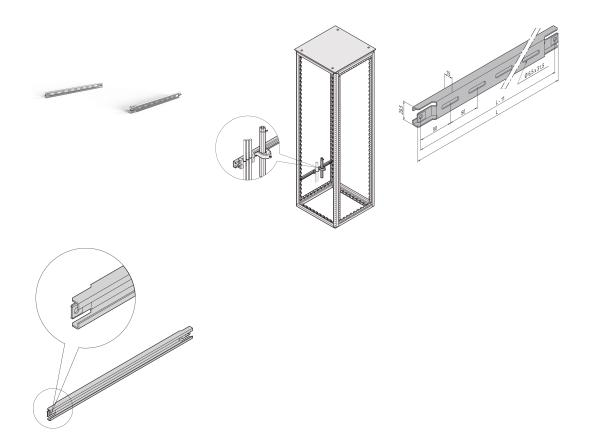
For cable ducting in side area of cabinet.
