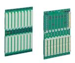
The nVent SCHROFF VMEbus Backplanes have outstanding high-frequency noise suppression and very high MTBF values due to ceramic capacitors and SMD fabrication technology.
