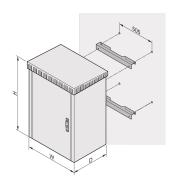
Unibody Wall Mounting Kit makes the double walled outdoor rack wall mountable. This function is used for in tunnel railways application and telecommunication applications.
