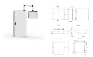
The mild steel operator interface control enclosure, OICE, has a pre-machined hole pattern to allow for the fixation to a swing arm, plus a removable front plate at an IP 55 protection degree. Components can be easily fitted thanks to the removable front plate, but will also be easily accessible through a rear door. Side handles on the enclosure allow for easy movement of the enclosure into the working position.
