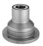
CS480 Swivel Base Bracket Coupling External mounts the enclosure directly to horizontal surfaces, enabling 340-degree enclosure rotation. Base mounting hardware is exposed. Maintenance-free bearings.
