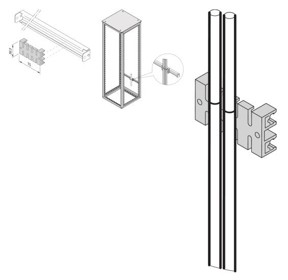
C-Rails are for better cable management. Installation generally behind the 19" uprights. They are compatible with standard cable clabs.
