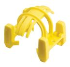
The nVent CADDY In-Wall Conduit Positioning Clip is an intuitive, tool-free and screwless solution to quickly and securely position 20 to 25mm conduits onto nVent CADDY Telescopic Screw Gun Box Straps. Ideal for drywall installations taking place before electricians arrive onsite to wire electrical boxes - commonly known as "hockey stick" installations.
