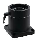
Syspend 281-Max Base Coupling attaches the enclosure directly to a horizontal surface. Enclosure can be rotated 300 degrees and locked in position. Includes safety stop and maintenance-free bearing.
