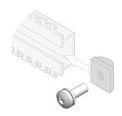
For variable assembly of 19" components outside the EIA increments
