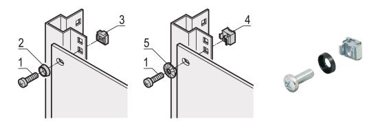
For standard grounding use a grounding nut and washer on at least one attachment point.
