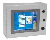
nVent RAYCHEM TraceTek TT-TS12 Touch Screen Panel provides a graphic user interface to manage and display information from a network of up to 250 external leak detection circuits. With interactive and dynamic leak location maps and displays, the leak location can be displayed on the floor plan, piping layout or photo of a single piece of equipment. Provides a quick status overview of all leak detection cables. Works with TTSIM or wireless mesh transmitters.
