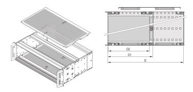
A cover plate is used for electromagnetic shielding or as mechanical protection.
