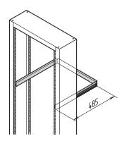
Labrack Cable Support Rail is designed for mobile 19" lab rack; with panel mounts also for stationary 19" lab rack. It allows smart cable management.
