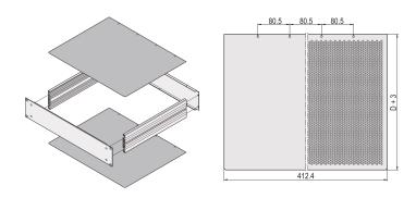
Cover plates plain will close the 19" chassis on top and bottom side. They protect the chassis from parts that could fall into the chassis.
