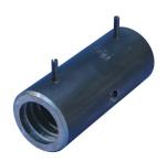
The side fill horizontal T-Series sleeve has vent holes located 90 degrees from the tap hole to facilitate side fill installations when the interferences of the structure will not allow top filling. Vent holes are added to horizontal sleeves to reduce air entrapment and help ensure proper filling of the sleeve.
