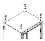
Bolt on lifting eyes to lift and place cabinet without cabinet damage.
