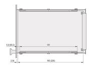
The guide rails can be clipped onto the perforated top / bottom cover. It is required if the PCB will be assembled from Slot 2
