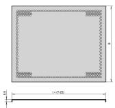
A cover plate is used for electromagnetic shielding or as mechanical protection. The cover can be used is non-standard boards will be assembled into the subrack.
