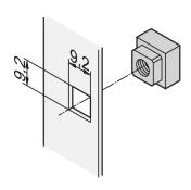
Square nuts have higher contact surface and dont get rounded off unlike hex nuts. For precise, anti-twist secure mounting without clearance, use square nuts.
