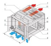
CompactPCI Desktop Chassis with vertical Card Cage for eight 3 U Boards, eight 3 U RTM Boards and one CompactPCI 3 U Pluggable Power Supply.
