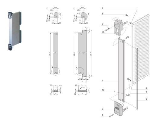
Plug-in unit, with IET inserter/extractor black handle, 3 U, front assembly. The U-shaped front panel enable shielding with a textile gasket.
