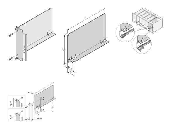
The air baffle with U-shaped front panel covers an empty slot to eliminate an air flow exit. The U-shaped front panel accepts a textile EMC gasket.
