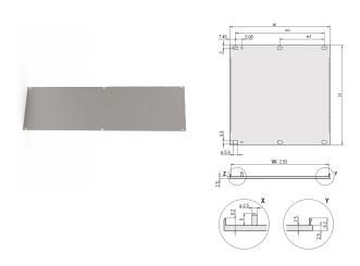
U-profile front panel for textile EMC gasket.
