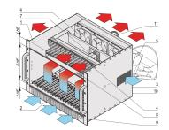
VME system for 21 VME boards 6 U, 160 mm. The power for the system is supplied by an open frame power supply. A fan control module monitors the fans, the temperature and voltage.
