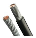
Theft-deterrent composite cables (TDCC) are conductors that function as copper conductors, but appear to be non-copper conductors and are difficult to cut and steal. These conductors are ideal for exposed electrical distribution grounding leads where copper theft may occur. Theft deterrent conductors are difficult to cut with hand tools and the outer steel stranding is magnetic, which further deters thieves looking for copper.
