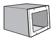
Cover with HMI cutout is secured to the front opening of ProLine Sloped-Front HMI Enclosure with semi-flush cover screws along the top and bottom cover edges. Use ProLine Frame Shelf or ProLine Grid Straps and Plates to support human-machine interface. Seamless foam-in-place gasket assures a watertight and dust-tight seal. It fits 500x600mm and 500Ax600mm ProLine Slope-Front HMI Enclosures.
