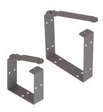
U-Connectors are used to rigidly join fittings to lay-in wireway straight sections. Top swings aside to retain the lay-in feature. One U-connector required at each wireway joint except telescope fittings, panel adapters, open adapters, closure plates or reducers.
