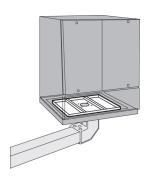
A Support Bracket is required when suspending a 600-mm wide ProLine Sloped-Front HMI Enclosure from above. The rigid bracket mounts inside the enclosure to stiffen its top. It can also be used inside a base for ProLine Sloped-Front HMI Enclosure when mounting from below. Bracket has prepunched holes to fit Compact Series 4 System 80 Flange Couplings as well as Swivel Tilts. Bracket is used as a template to drill holes in the enclosure.
