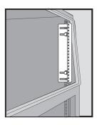
Symmetrical Rack Angles have through-holes in mounting surfaces for mounting rack equipment. Rack Angles with through-holes accommodate either English or metric cage nuts
