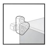
Mounting Bracket Kit has four polycarbonate brackets and four M4 self-tapping, plated screws. Kit is field-installable. Use on all QLine D enclosures. Maintains listed ratings for enclosure.
