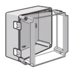
Hinge Kit includes two polyamide hinges, eight M4 self-tapping, plated screws, eight flat washers and drilling templates. Use on all QLine D enclosures; meets Type 4 requirements. Use on QLine E enclosures; kit is not guaranteed to meet Type 4 requirements, and should be reviewed by customer.
