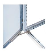
The Door Stop Kit holds doors open at 130 degrees. The kit includes a slotted bracket that mounts to either the top or bottom of the door and a stop arm that attaches to the frame.
