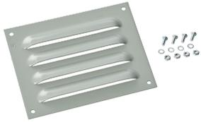
Designed to provide ventilation in enclosures where excessive internal heat or excessive moisture is a problem. These kits may be easily installed in the field by making a cutout of the proper size and attaching the louver plate in place.
