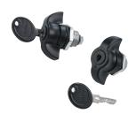
The Keylocking Quarter-Turn Wing Knob locks a variety of wall-mounted enclosures. The Wing Knob includes a gasket, mounting nut and one key with the 333 key code. This Wing Knob should be used with an existing cam for installation; please note the cam is not included with Wing Knob. It can be locked in the open or closed position. This product maintains the cabinet rating Type 4, 12.
