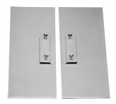
Enclosure Stabilizers help prevent injury to workers by stabilizing floor-mount enclosures which are not bolted down. To install, slip the stabilizer under the floor stand and tighten two thumb screws.
