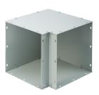
Lay-in Painted 90-Degree Elbows have all removable sides, retaining lay-in feature regardless of how the elbow is oriented. Lay-in feature allows wires and cables can be laid in along wireway run. No pulling through of wires or cables prevents damage to insulation that often occurs in a pull-through wiring system. Sides are held together with screws.
