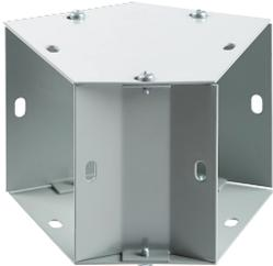
Lay-in Painted 45-Degree Elbows are used for continuous run with 45-degree turns. Top and inside covers removable so wires and cables can be laid in along wireway run. No pulling through of wires or cables prevents damage to insulation that often occurs in a pull-through wiring system.
