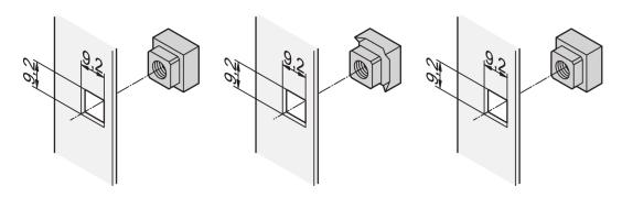
Square nuts have higher contact surface and dont get rounded off unlike hex nuts. For precise, anti-twist secure mounting without clearance, use square nuts.
