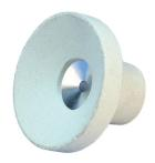
The ceramic insert and disk fit inside the pouring basin crucible and are intended to retain the filler material until the exothermic reaction is complete and melts the disk. Once the disk has melted, it allows the molten filler material to gravity feed the pouring basin.
