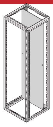
Varistar Mounting Plate for mounting electrical components and sub-assemblies, with 600 kg load capacity. The mounting plate can also be rear mounted and strengthening bracket can be added to increase load capacity.
