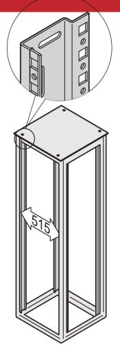
Varistar ETSI 23" rack for housing telephone (primarily), computer, audio, and other equipments. It is compatible with the Slim-Line Frame.
