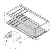
Mounting plate for heavy components or proprietary electronic assemblies. Suitable for RatiopacPRO/-AIR, CompacPRO and EuropacPRO.
