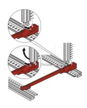
The the standard type guide rail with connector fixing allows the user to clip the DIN connectors (EN 60603-2 (DIN 41612)) directly onto the guide rails. Only applicable with Euroboards with the dimensions 100 x 160 mm and 100 x 220 mm. Suitable for RatiopacPRO/-AIR, PropacPRO, CompacPRO and EuropacPRO.
