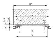
Guide rail mid-piece for individual multi-piece guide rails out of plastic or Aluminum extrusion. Suitable for Standard, Acessory, 4.4" PCB types and end pieces with coding.
