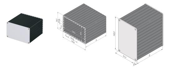
The rectangular Alu-profile case enables a user to insert 4 standard PCBs (height 100 mm x depth 160 mm). The PCBs will be inserted in grooves in the Alu-profile tube. Both sides are covered with 2.5 mm thick front panels.
