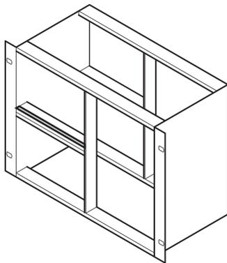
The contact strip makes contact between horizontal rails. If two horizontal rails are mounted one above the other, the seals plus a metal strip enable EMC shielding.
